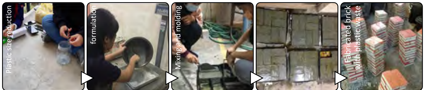
Fig. 1 The fabrication of eco-brick paver at Civil Engineering Concrete laboratory of UMS.
